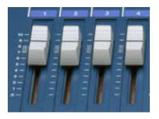
The Tascam's white Channel Faders will access both the CEP Mixer Window Track Faders as well as the Track Volume value in the Track Controls area of CEP (at the left of each track). The Tascam's four Channel Faders are governed by a BANK switch.
